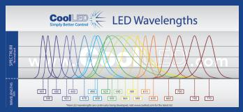
20 different LED wavelengths from the near-UV at 365 nm to the near-IR at 770 nm
