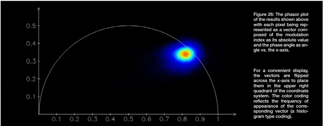
Very often both luminescence lifetime distributions differ from each other, which can be a hint for the presence of multiple lifetimes as described in literature. Generally, the modulation index signal is more noise dependent than the phase angle signal.
