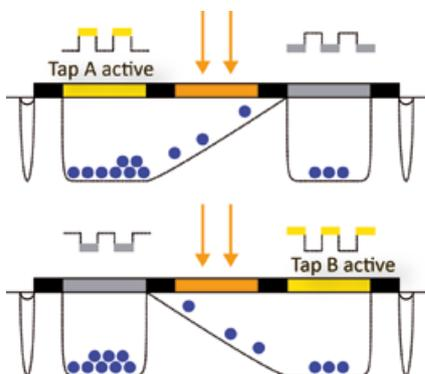
Figure 16: Schematical drawing<sup>3</sup> of the in-pixel charge swing of the QMFLIM2 image sensor.
