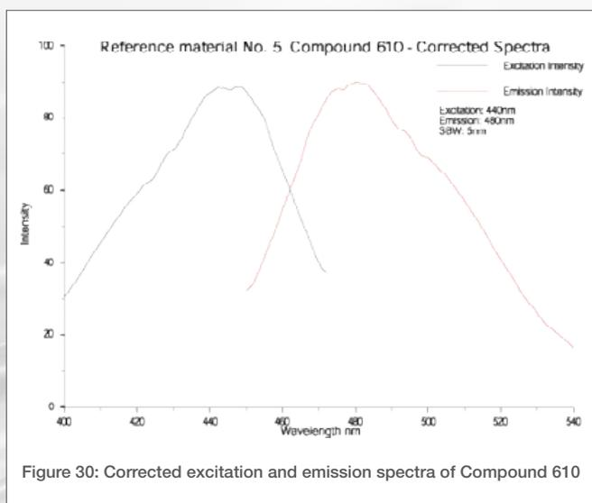
Figure 30: Corrected excitation and emission spectra of Compound 610
