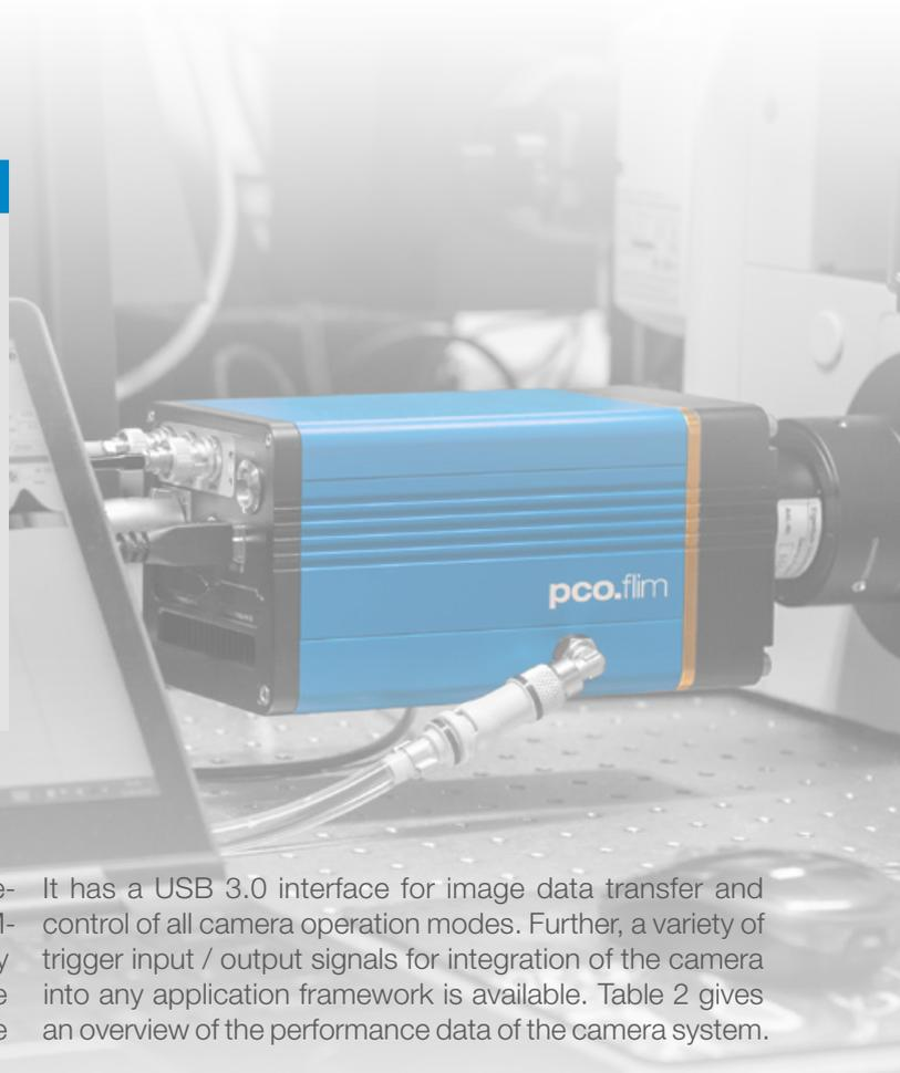
The pco.flim camera system is the first luminescence lifetime imaging camera using the CMOS image sensor QM-FLIM2. It offers all the required generation of frequency domain signals (5 kHz – 40 MHz) and also allows the use of external modulation signals in a limited frequency range (500 kHz – 40 MHz).
