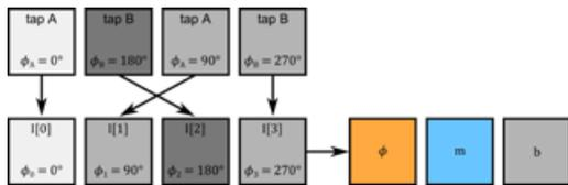
In the above figure the top row shows the sequence order of phase images out of the camera. The phase images have to be (virtually) re-sorted to an ascending phase sequence for the computation of the phase, demodulation index and intensity images (bottom row).
