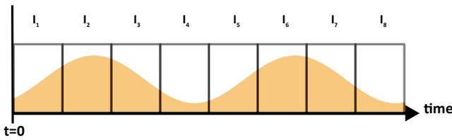
Figure 12: Sinusoidal luminescence signal (orange) with four sampling integration windows per period (grey rectangles), where the integrated light results in the intensity images  $I_1 \dots I_8$  ( $I_5 \dots I_8$  are the repetition of  $I_1 \dots I_4$ )
