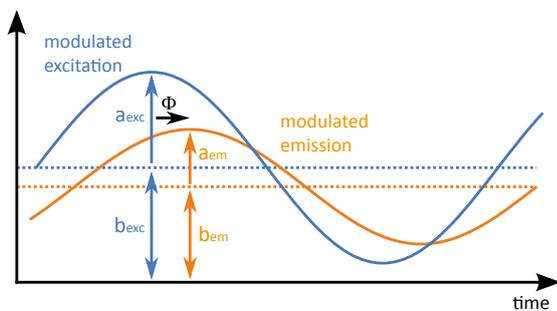
Figure 10: Time responses of excitation light (blue) and luminescence (orange) emission if luminescence lifetime imaging is done in frequency domain (extract from continuous signals). Amplitudes  $a_{exc}$  and  $a_{em}$ , constant or direct components  $b_{exc}$  and  $b_{em}$  and phase angle or phase shift  $\Phi$  are denoted.
