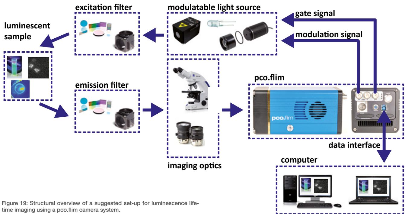
Figure 19: Structural overview of a suggested set-up for luminescence lifetime imaging using a pco.flim camera system.
