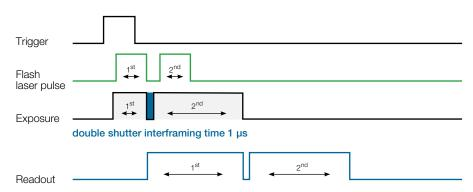
The duration of the first exposure time can be configured. The duration of the second exposure time is fixed and pre-defined by the readout time of the first image. Therefore, it is usually necessary to prevent the sensor from ambient light during the prolonged second exposure time.
