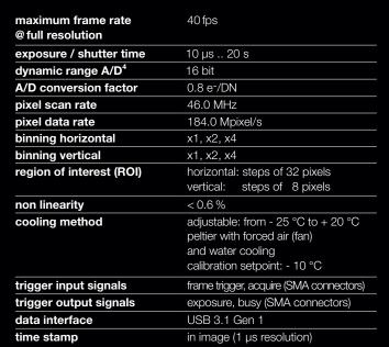
$<sup>^4</sup>$  The high dynamic signal is simultaneously converted at high and low gain by two 12 bit A/D converters and the two 12 bit values are sophistically merged into one 16 bit value.
